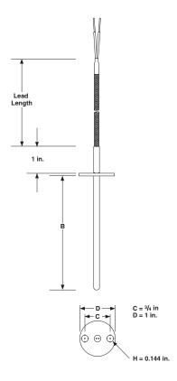
The flanged thermocouple allows rapid assembly and low profile when going through bulkheads.
