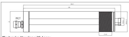
**Electronics Housing with Laser**
