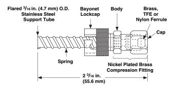
This fitting combines the features of the fixed bayonet fitting in a compact unit which does not require brazing to assemble.
